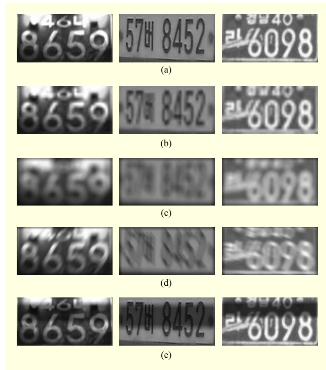
Fig. 2. Sample images in test database, including (a) original, (b) downsampled, (c) Gaussian blurred, (d) motion blurred, and (e) shadowed.
