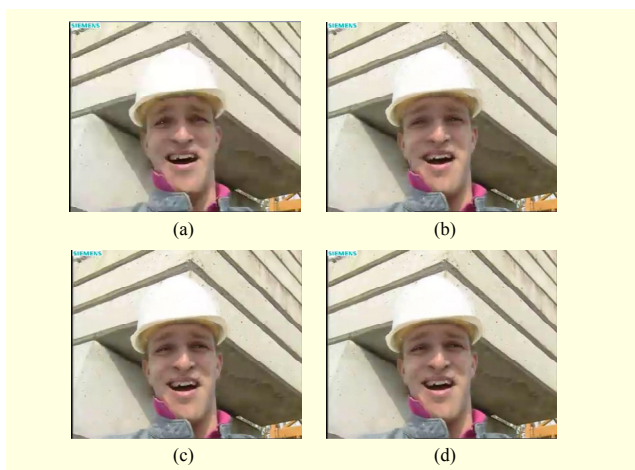
Fig. 12. Subjective quality comparison: (a) BLskip with 0.005% coding complexity and PSNR=32.40 dB, (b) proposal with 0.1% coding complexity and PSNR=32.90 dB, (c) proposal with 10% coding complexity and PSNR=33.35 dB, and (d) JSVM with 100% coding complexity and PSNR=33.40 dB.
