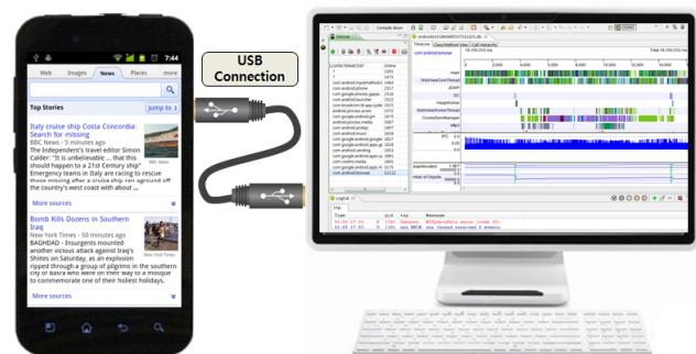
Fig. 15. Android phone used for experiment and analyzed result of web browser application by AndroScope. AndroScope view is matched with left side of Fig. 13.
