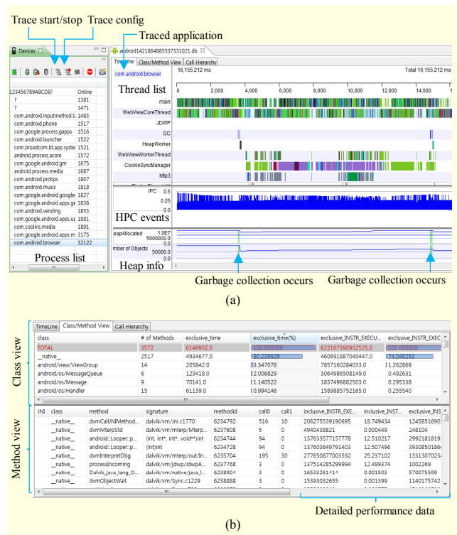
Fig. 13. Screenshot of advanced Traceview integrated into DDMS: (a) trace interface and timeline view and (b) profile view.
