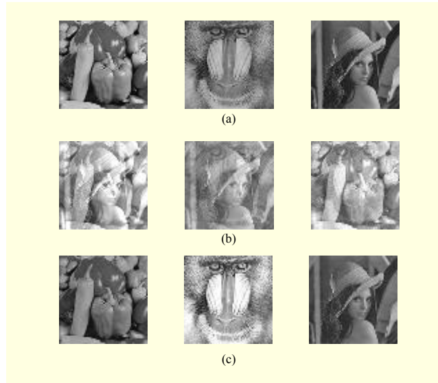
Fig. 3. Image separation for proposed EG-NICA algorithm, showing (a) three source images, (b) three mixed images, and (c) three recovered images.
