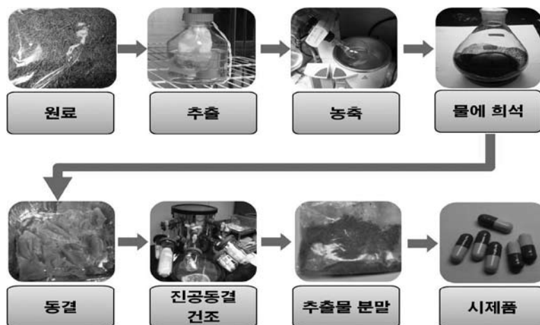
Fig. 13. Manufacturing procedure of natural sleep aids by ethanol extraction
