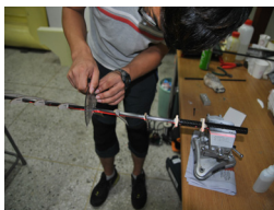
Figure 7. Pitch angle check
