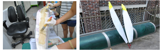
Figure 9. Covered glass fiber Figure 10. Completed propeller
