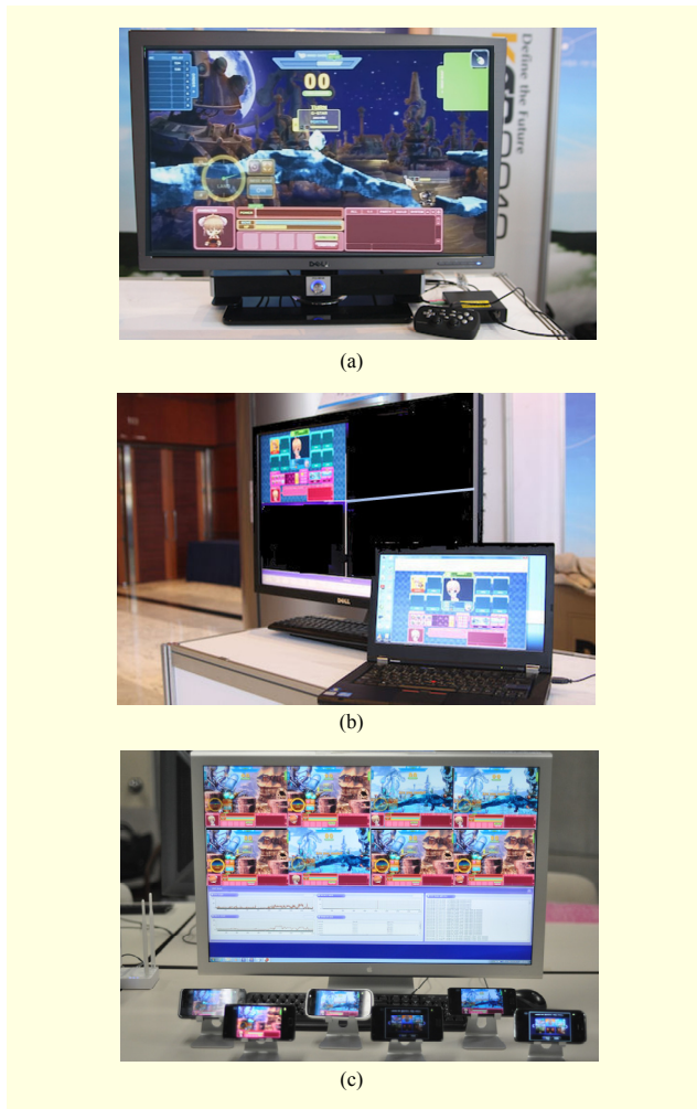
Fig. 7. Game service platform supporting multiple users and devices: (a) set-top box (1080 p) connected to one user, (b) tablet PC connected to four users, and (c) smart mobile devices connected to eight users.
