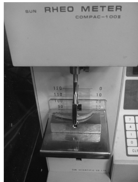
Fig. 3. Cutting test of the melon stem.
