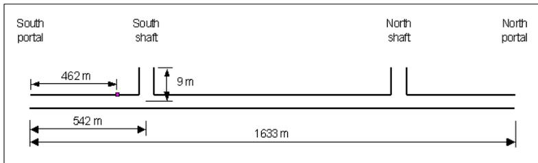
Fig. 3. Schematic diagram of tunnel
