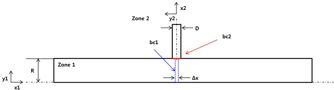
Fig. 1. Axisymmetric Computational Domain of Tunnel and Vertical Shaft
