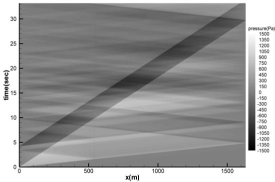
Fig. 12. Tunnel wall x-t diagram (one shaft)
