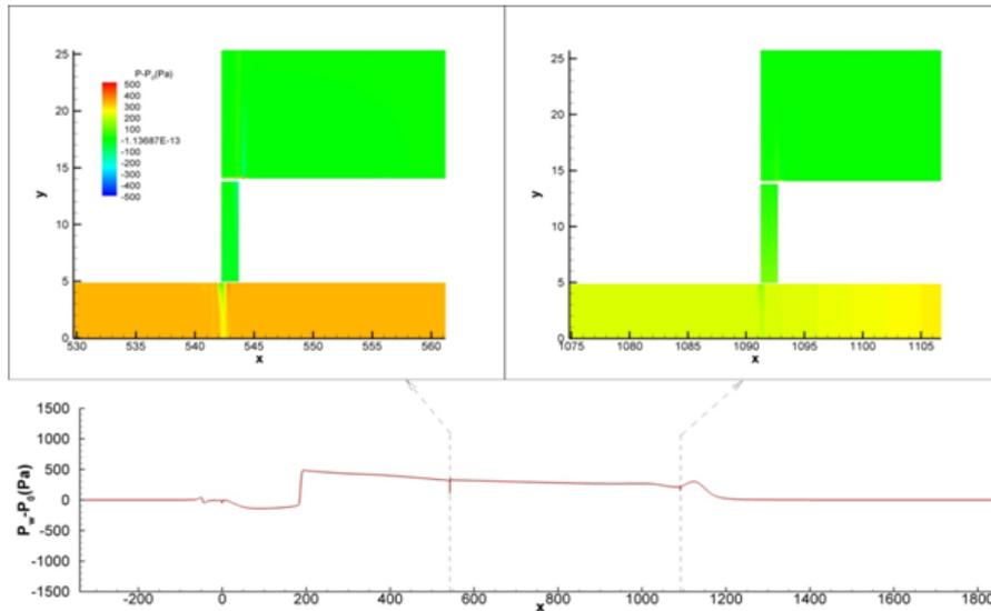
Fig. 16. Pressure distribution on tunnel wall and air shaft (t=3.40sec)
