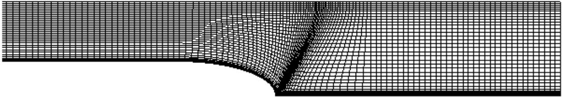
Fig. 8. Grid around train nose (zone1)
