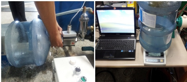
Figure 23. Measurement of measured amount of the disinfectant sprayed.
