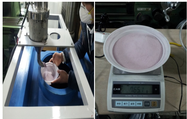
Figure 27. Measurement of controlled screw conveyor pump amount.
