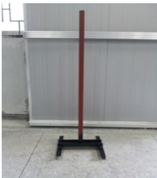
Figure 8. The pedestal for attachment of water level sensor.
