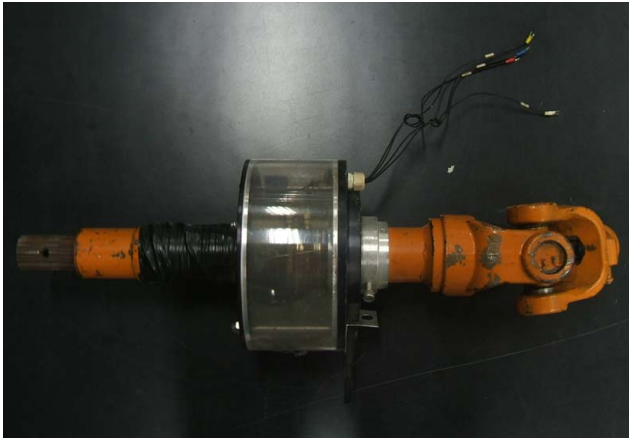
Figure 2. Picture of the torque meter used in the test.
