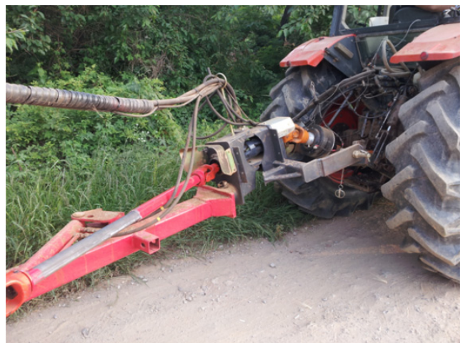
Figure 4. Connection of PTO power measurement.
