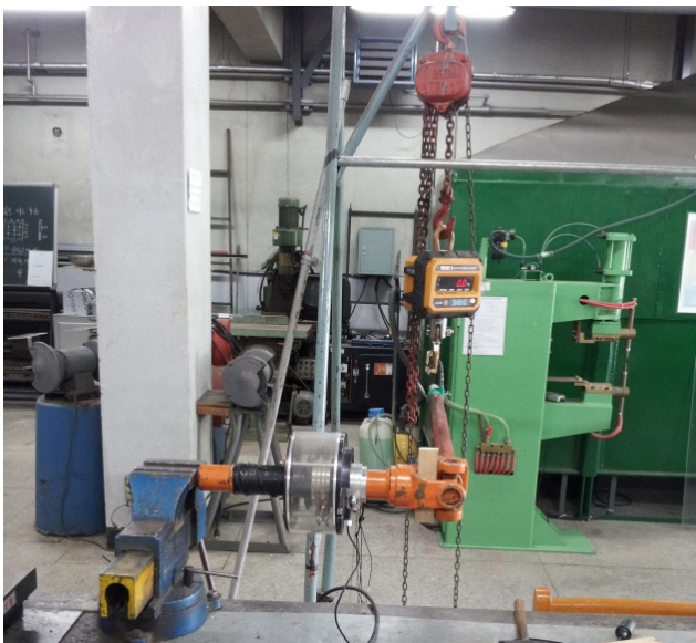
Figure 3. Calibration test of the torque meter.
