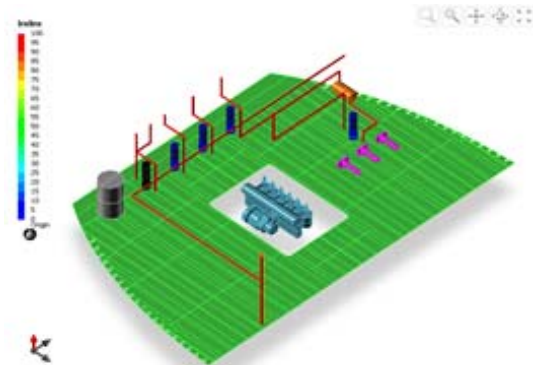
Figure 9: Pipe Arrangement of Deck 1
