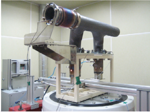
Figure 11: Test rig to simulate thermal and vibration movements
