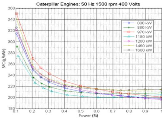
**Figure 3:** Diesel generator SFC curve[6]
