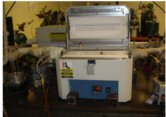
(d) Furnace with installed Cu-Chabazite sample
