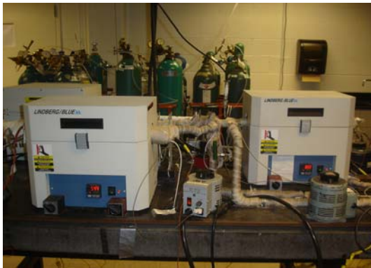
(c) View of steam generator and furnace for SCR
