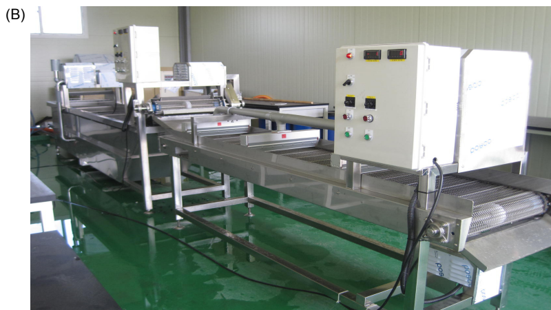
Fig. 1. A schematic view (A) and a photo (B) of bubble-aqueous chlorine dioxide washing system. ① bubble washer main frame, ② washing supply plate, ③ waterwheel, ④ waterwheel motor, ⑤ washing blower, ⑥ washing conveyer belt, ⑦ washing conveyer motor, ⑧ washing discharge plate, ⑨ control box, ⑩ dehydrator main frame, ⑪ dehydrating conveyer belt, ⑫ dehydrating conveyer motor, ⑬ dehydrating air knife, ⑭ air jet pipe, ⑮ blower, ⑮-1 dehydrating discharge plate, ⑮-2 control box.
