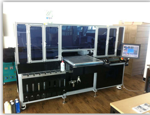
Fig. 6. Multi-pass, laboratory ink-jet printing system for ceramic tiles in KICET.
