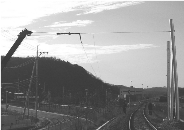
Fig. 8. Real scale load test for pole foundations(KRRI, 2010)
