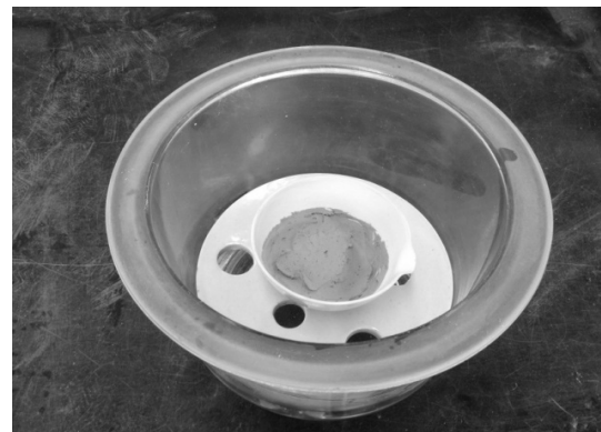
Fig. 3. Soil container for undrained shear strength at liquid and plastic limit states
