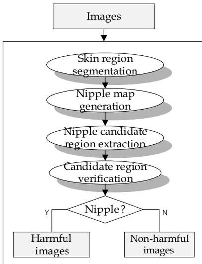
[Fig. 1] Overall flow of harmful image detection
