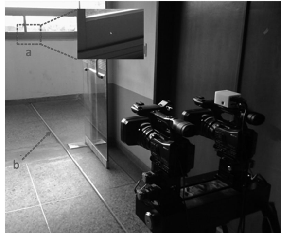
Fig. 7. An accuracy test of the fabricated laser sensor module on the 3D camera rig: (a) Laser beam and (b) tape measure.
