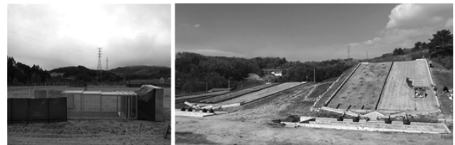
Fig. 2 Portable wind erosion tunnel test and land with a slope of 20° on test site
