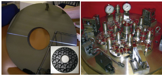
Fig. 1 Configuration of SiC light-weight mirror machined by ELID grinding technology and jig of static pressure supporter
