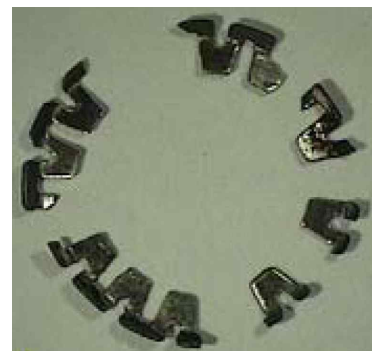
Fig. 5 The fracture of lock-claws after fatigue test (2)
