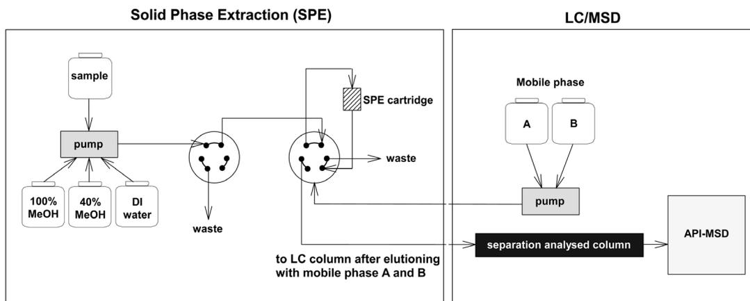
Fig. 1. Schematic diagram of the on-line SPE-LC/MSD.<sup>41)</sup>
