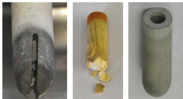
Fig. 3. Electrodes after Testing in Molten Salt (Left to Right): Sr Sensor Shattered (shown with Outer Housing), K Sensor with Major Damage, Intact Na Sensor.
