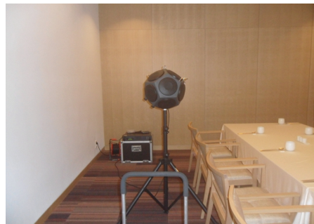
Fig. 3 Measurement scene and noise generator system
