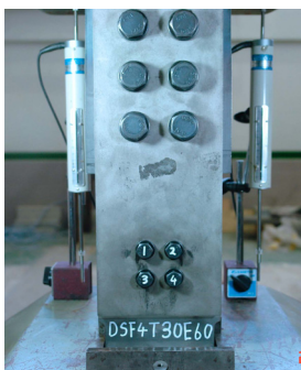
Fig. 4 Set up of specimen and transducer (LVDT) for 2×2 bolt array
