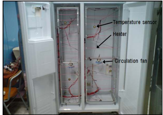
Fig. 1. Photograph of electric heating system and temperature sensors installed inside the refrigerator.
