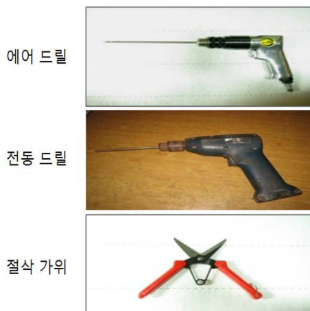
Fig. 3. Representative tools for dismantling waste flat panel displays.
