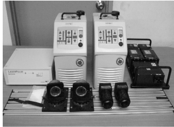
Fig. 5. 3-dimensional PIV system
