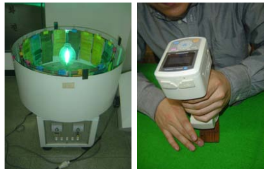
Fig. 1. Fading test setup (left) and spectrophotometer (right).
