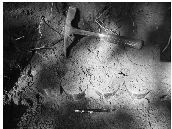
Fig. 3. Soil sampling method from the natural terrain
