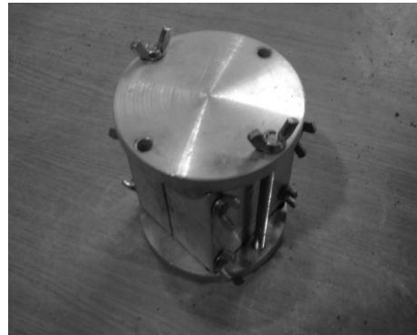
Fig. 2. Specimen Preparation Mold for Unconfined Compressive Strength Tests
