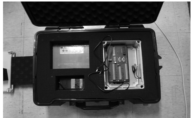
Fig. 8. Datalogger and battery system
