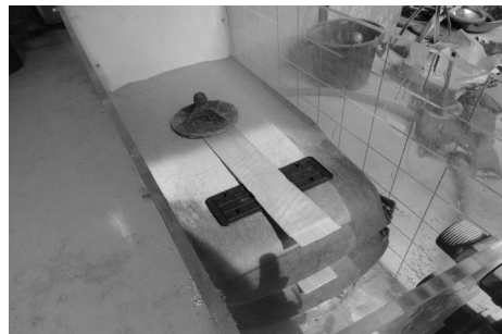
(b) Stacking second soilbag, installation PBD
