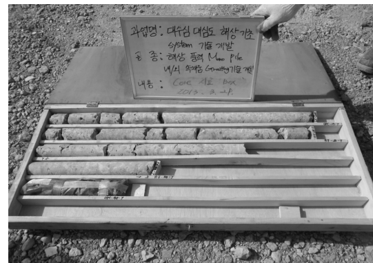
Fig. 5. Boring core sampling
