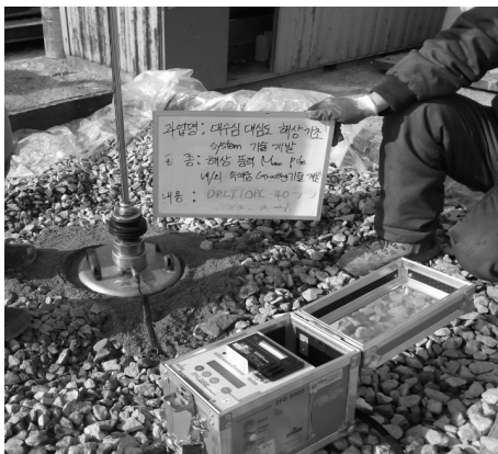
Fig. 10. Panoramic view of dynamic plate load test
