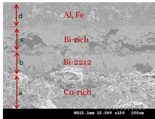
Fig. 4. The cross-section SEM image of the ABAB coating layers out of substrate/Al 2 O 3 /ABAB/Al 2 O 3 /substrate plasma coating specimen after PMP-AT (5 hr) in air.
