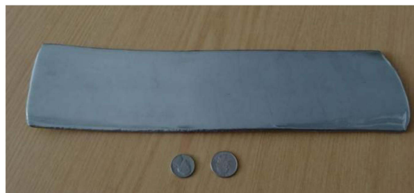
Fig. 4. Photo of a Hot-rolled Specimen L-350xW-90xT-6 [mm]
