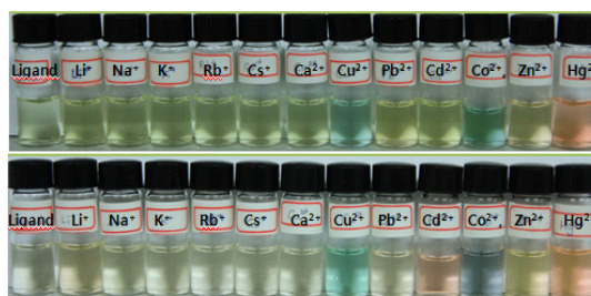
Fig. 1. Colorimetric change in the color of 1 \times 10^{-5} M solution of 1 (above), 2 (below) with 8 equivalents of the metal ion.
