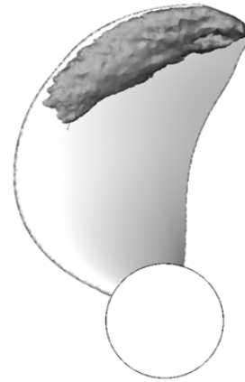
Fig. 14 Cavity on KP505 propeller blade
