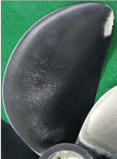
Fig. 16 Cavitation erosion on propeller blade[22]
