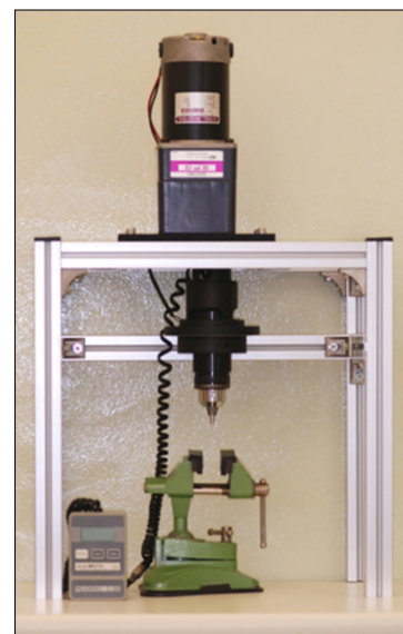
Fig. 6. Removal torque value measuring set. This is composed of a digital torque gauge, a specimen loading apparatus, an aluminum framework, and specimen grip device.
