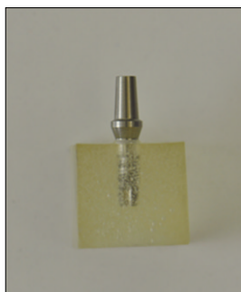
Fig. 5. Specimen preparation. Implant fixture to resin block is fixed. Then connect abutment and abutment screw.
