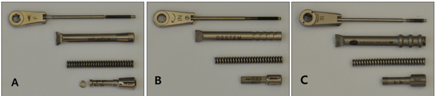
Fig. 1. Mechanical Torque-Limiting Devices (MTLDs). From top to bottom, head, body, spring, handle. A: Dentium MTLD, B: Osstem MTLD, C: Shinhung MTLD.
