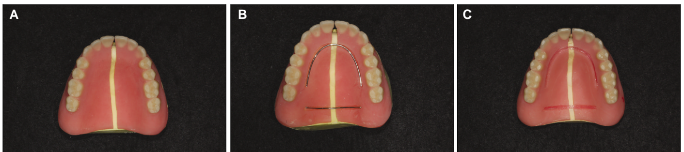
Fig. 2. Location of reinforcement materials in midline fracture of maxillary complete denture. A: without reinforcement (control group), B: with metal wire reinforcement (group W), C: with glass fiber reinforcement (group G).
