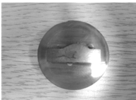
Fig. 1 Welding output section
