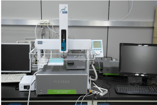
Fig. 2. Commercial laser spectrometer (CRDS from Picarro) used in this study.
