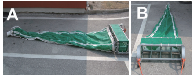
Fig. 2. Rectangular bottom net to collect larvae and juveniles used in this study. A: side view; B: front view.
