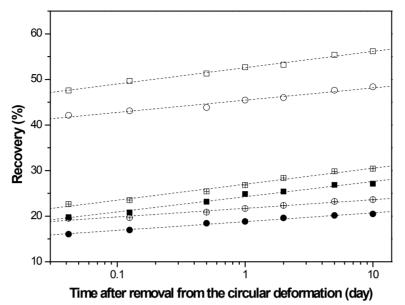
**Figure 5.** Recovery variations from the circularly deformed sample after thermal aging at 90°C with the measurement time. The squares and circles indicate the aging medium systems of the air to water ( $A \rightarrow W$ ) altering system and the water to air ( $W \rightarrow A$ ) altering system, respectively. The open, solid, and crossed symbols denote the filler systems of unfilled, carbon-filled, and silica-filled systems, respectively.
