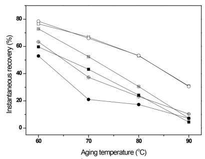
**Figure 7.** Variations of the instantaneous recoveries at  $10^{-6}$  day with the aging temperature. The squares and circles indicate the aging medium systems of the air to water (A $\rightarrow$ W) altering system and the water to air (W $\rightarrow$ A) altering system, respectively. The open, solid, and crossed symbols denote the filler systems of unfilled, carbon-filled, and silica-filled systems, respectively.
