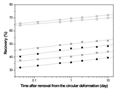
**Figure 4.** Recovery variations from the circularly deformed sample after thermal aging at 80°C with the measurement time. The squares and circles indicate the aging medium systems of the air to water ( $A \rightarrow W$ ) altering system and the water to air ( $W \rightarrow A$ ) altering system, respectively. The open, solid, and crossed symbols denote the filler systems of unfilled, carbon-filled, and silica-filled systems, respectively.
