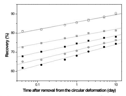
**Figure 2.** Recovery variations from the circularly deformed sample after thermal aging at 60°C with the measurement time. The squares and circles indicate the aging medium systems of the air to water  $(A \rightarrow W)$  altering system and the water to air  $(W \rightarrow A)$  altering system, respectively. The open, solid, and crossed symbols denote the filler systems of unfilled, carbon black-filled, and silica-filled systems, respectively.
