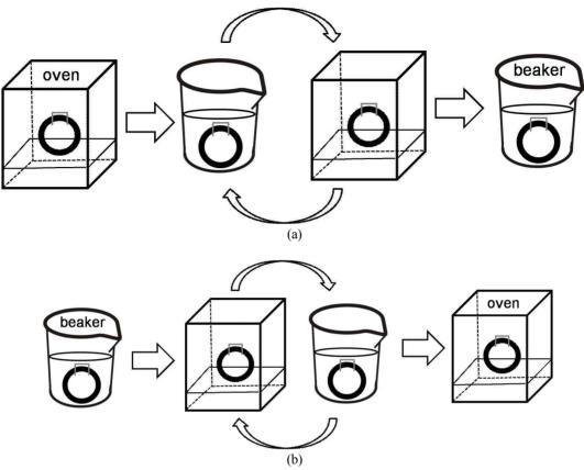
Figure 1. Altering aging medium systems of the circular deformation test. (a) the air to water altering system (A $\rightarrow$ W altering system, changing the medium each one day, the initial medium was air) and (b) the water to air altering system (W $\rightarrow$ A altering system, changing the medium each one day, the initial medium was distilled water).
