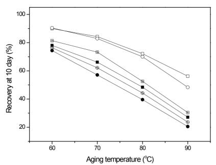
**Figure 6.** Variations of the limited recoveries (recoveries at the measurement time of 10 days) with the aging temperature. The squares and circles indicate the aging medium systems of the air to water  $(A \rightarrow W)$  altering system and the water to air  $(W \rightarrow A)$  altering system, respectively. The open, solid, and crossed symbols denote the filler systems of unfilled, carbon-filled, and silica-filled systems, respectively.
