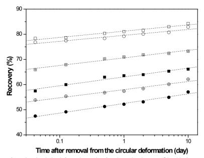
**Figure 3.** Recovery variations from the circularly deformed sample after thermal aging at 70°C with the measurement time. The squares and circles indicate the aging medium systems of the air to water ( $A \rightarrow W$ ) altering system and the water to air ( $W \rightarrow A$ ) altering system, respectively. The open, solid, and crossed symbols denote the filler systems of unfilled, carbon-filled, and silica-filled systems, respectively.
