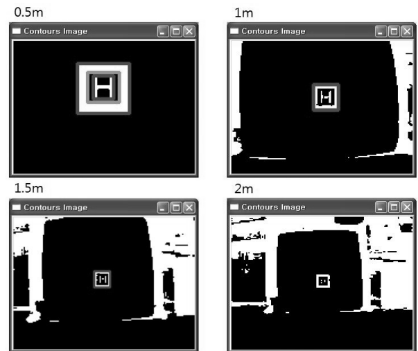
Fig. 14. The marker image displayed on the mock-up AGV with respect to the relative distance from the mock-up AGV to the marker
