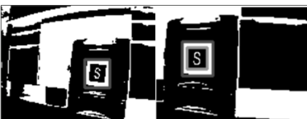
Fig. 9. The extraction of the candidate region for the marker(left) and its verification(right)
