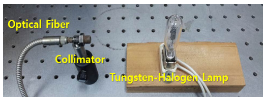
Fig. 4 Photograph of calibrated tungsten-halogen lamp measurement.
