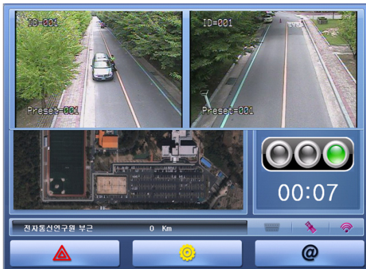
Fig. 2 Display example of intersection safety supporting service and traffic light information service.
